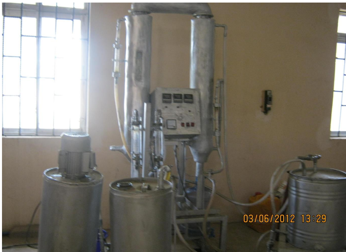
Figure 1: Continuous Oscillatory Baffled Reactor Arrangement (COBRA)
